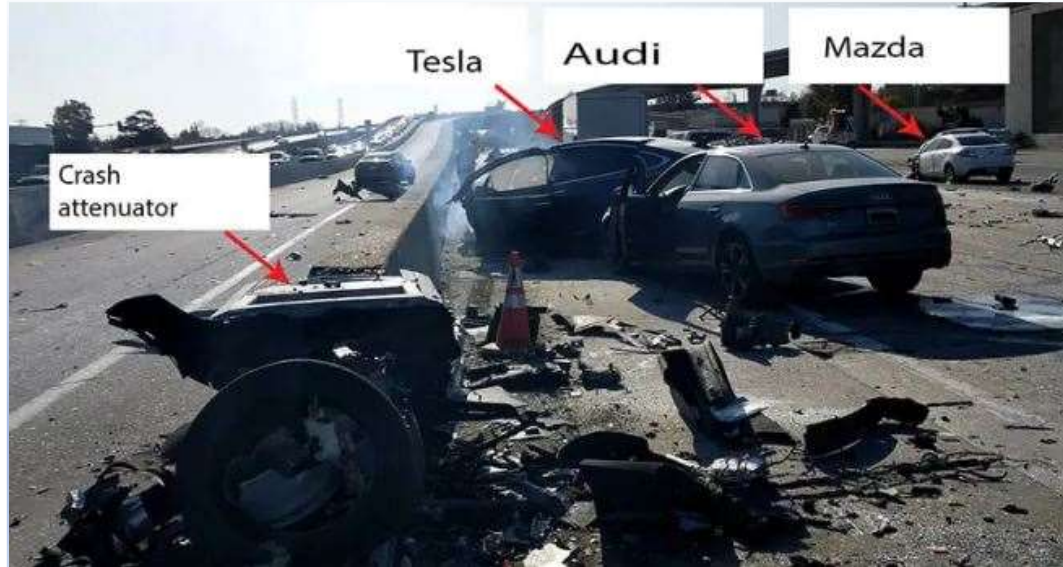
7 8 9 10 11 12 13 14 15 16 Fatal 2018 crash involving Autopilot, in which Tesla's software suddenly steered the Tesla to the left, directly into a concrete barrier on a highway in Mountain View, California. Photograph by NTSB.
